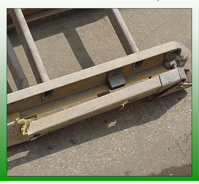
• Defective ladder must be marked or tagged.
