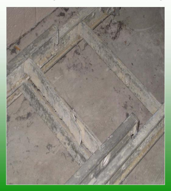
Defective ladders with broken side rails must be removed from service until repaired.
